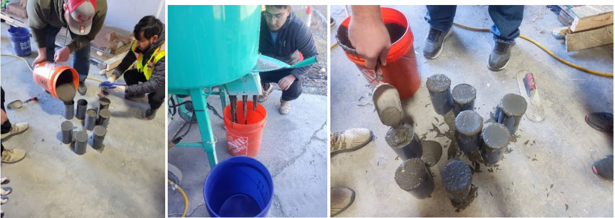
Mixing and Sampling UHPC
