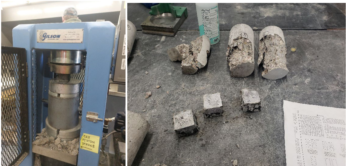
Testing UHPC Concrete Samples for Compressive Strength
